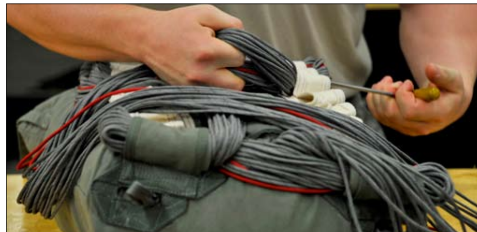
Petty Officer 2nd Class Joshua Goldsmith, United States Special Operations Command Central parachute rigger, secures a deployment bag to a canopy during parachute packing at MacDill, Sept. 18. Parachute connections are made using quarter-inch cotton webbing and are secured by tying a surgeon's knot.
