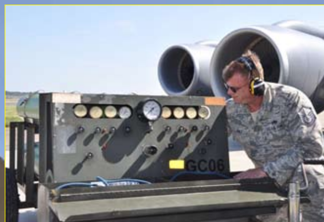
Master Sgt. Thomas Cole, 927th Aircraft Maintenance Squadron, services the oxygen system of a KC-135 Stratotanker prior to departing for MacDill Air Force Base, Fla. from Royal Air Force Mildenhall, England, April 16.
